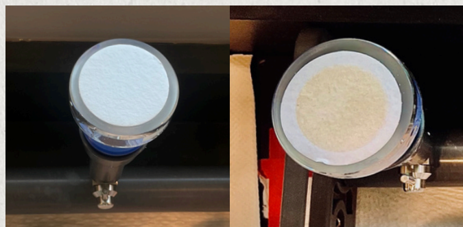
Figure 3: Before and after filtering water samples for chlorophyll-a. Glass fiber filters are typically white and snowy in appearance (left); following filtration, the filter has “trapped” the sample, typically resulting in a yellowish or green color.
