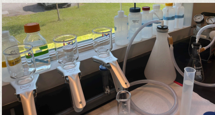
Figure 2: Filter apparatus and vacuum pump setup. Our filter apparatus can process three samples with one vacuum pump, making processing Wallenpaupack Monitoring samples faster!
